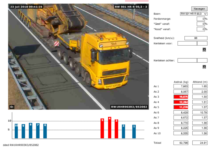
Figure 2: WiM software showing sensors recording a passing truck.
