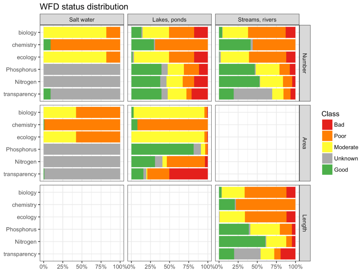
Figure I.11 Percentage of area of open water bodies in the Netherlands with bad (red), poor (orange), moderate (yellow), good (green), very good (blue) biological quality, chemistry, ecological quality, total P, total N and transparency. Depicted per water body or water course (top row), based on area of the water bodies (middle row) and based on length of the water courses (bottom row).
